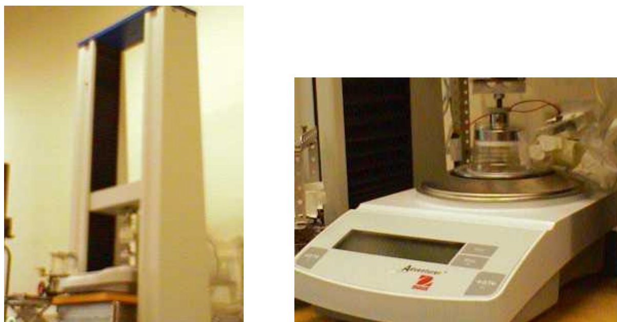
Figure 2: Universal testing machine modified to perform compression experiments on cylindrical soft tissue samples. The left side shows an overview of the machine with integrated balance, the right hand side gives the balance with climate chamber and piston.
